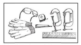
**Step 1: Tools needed**Plastic scoring tool, tape measure, clamps, straight edge, safety glasses and gloves.
