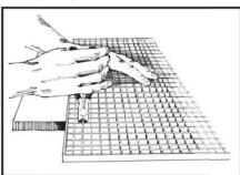
**Lighting Louvers:**Snip off excess with diagonal cutters.
