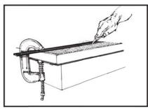
Step 2: Measure & Score Measure, clamp straight edge, lightly pull scoring tool across the smooth side of the panel, repeal until 1/2 through.
