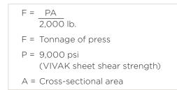
Cross-sectional area is determined by the perimeter of the object to be cut times the thickness of blade penetration.
