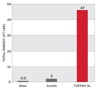
\*Instrumented Impact per ASTM D 3763, sample thickness 0.125" nominal
